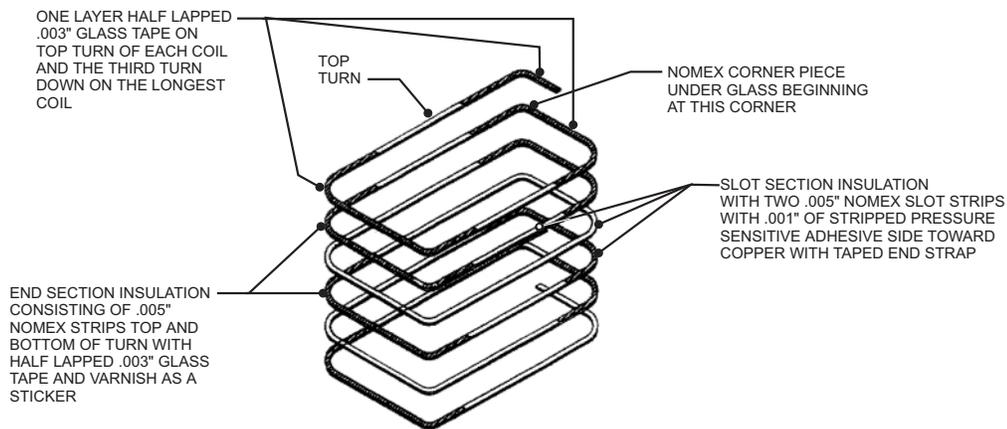
**Figure 17.** Taped and strip insulation system
