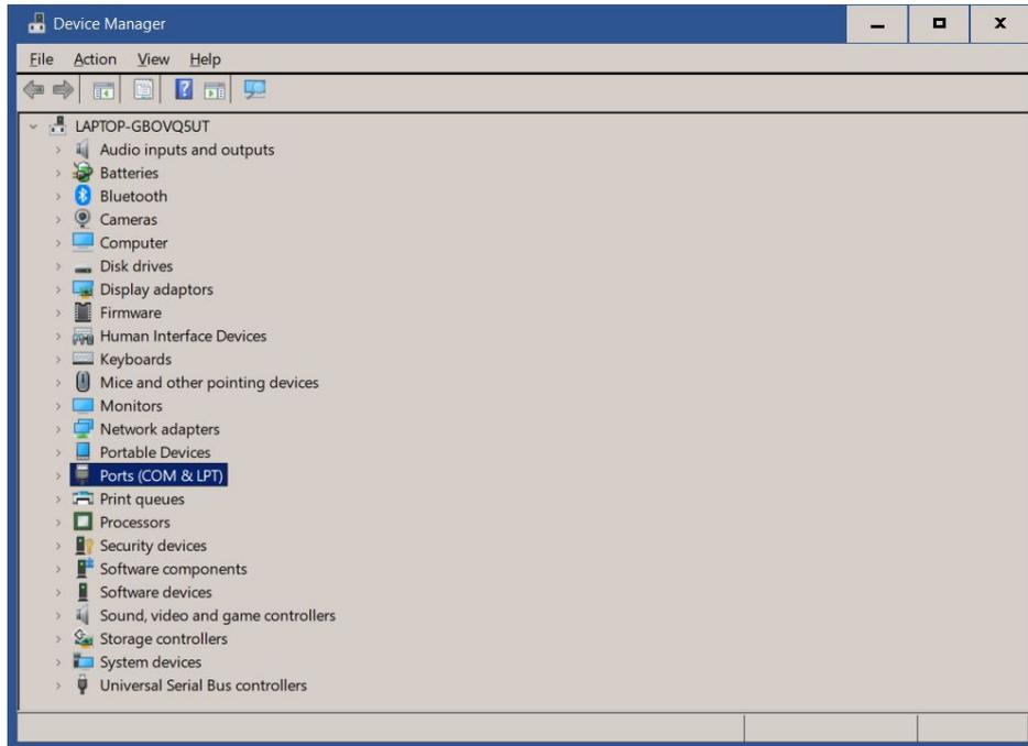
Now expand the **Ports (COM & LPT)** option by clicking on the > arrow. The list of com ports in use is displayed (in this case, COM3 as shown below).
