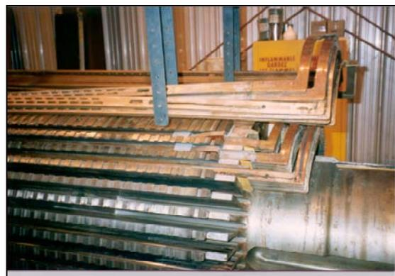
Fig. 2 Typical field winding showing both the middle and end sections. Some of the turns are shown lifted from the slots.
