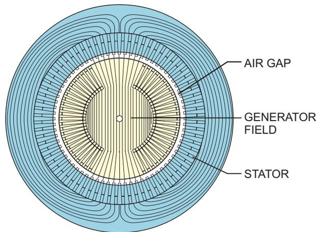
**Figure 4.** Rotor magnetic flux linking rotor and stator
