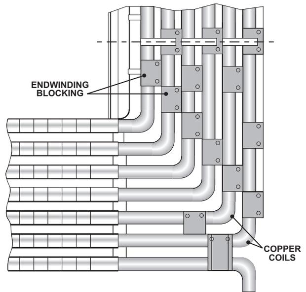
**Figure 19.** Endwinding blocking
