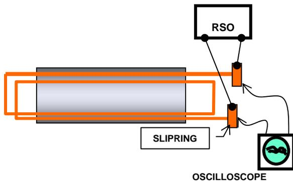
Fig. 4 RSO test arrangement
