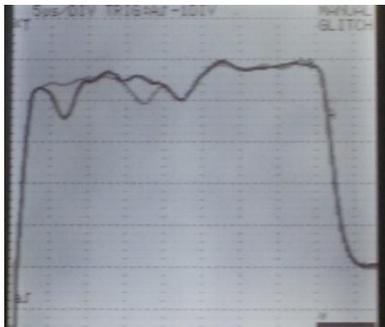
Fig.8 Waveform with inter turn short
