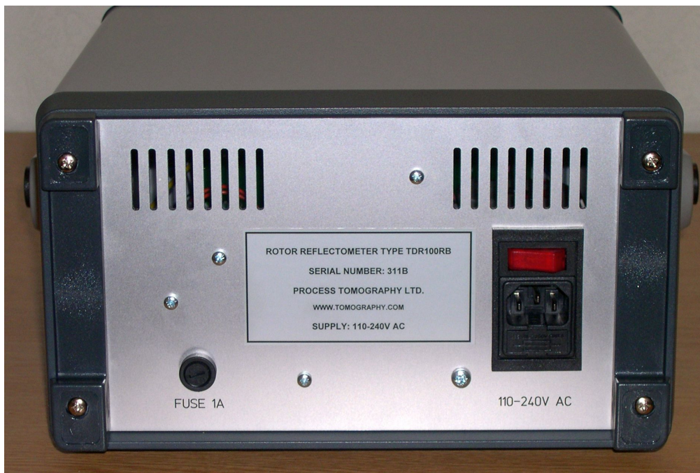
REAR VIEW SHOWING MAINS INPUT AND BATTERY FUSE HOLDER
