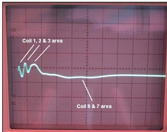
Fig. 8 RSO trace showing multiple shorted-turns
