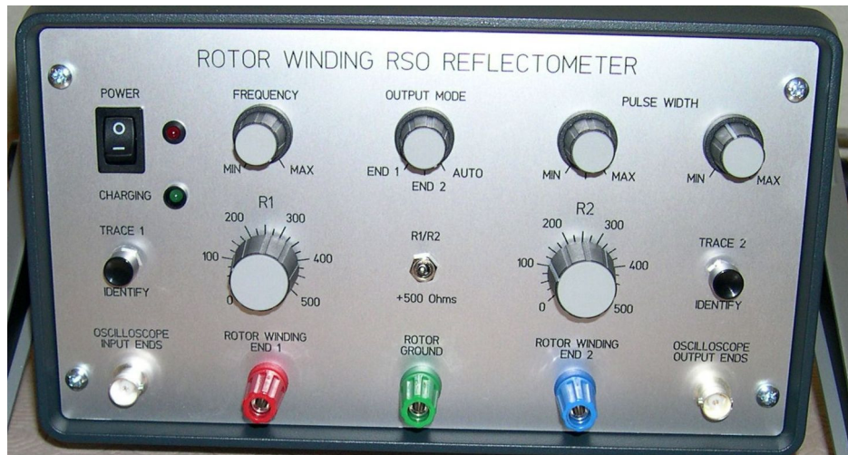
Figure 2.4 Reflectometer front panel controls (TDR100RB)
