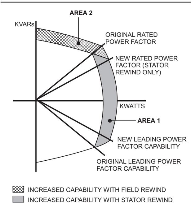
**Figure 20.** Uprating capability curve
