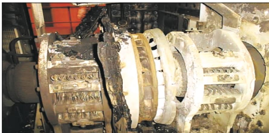
**Figure 12.** Collector and brush holder neglect
