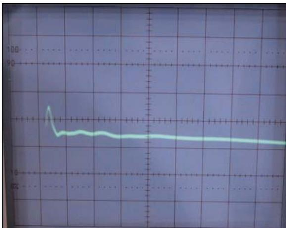
Fig. 7 The waveform shows the summed up signal from a rotor with a shorted-turn.
