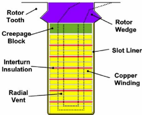
Fig. 3 Cross-section of a cylindrical rotor slot showing the winding conductors and insulation
