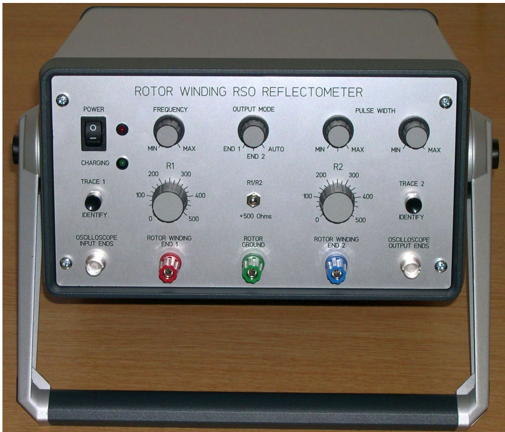
FRONT VIEW OF TRDR100RB ROTOR REFLECTOMETER
