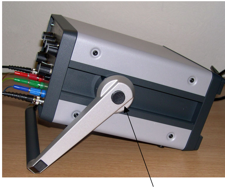
Figure 2.9 Handle pivot buttons (one on each side)
