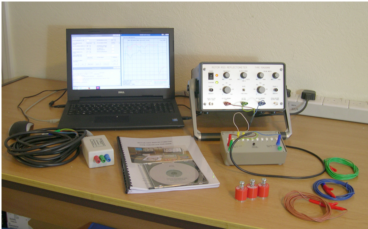
The TDR200 RSO Rotor Reflectometer measurement system
