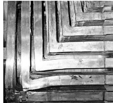
Fig.11 Typical shorted turns of rotor winding
