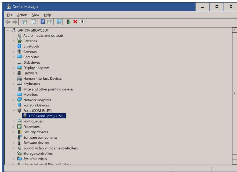
If only one port is shown, as in the case above) this is the comport number in current use (**COM3**). This number should be entered in the comport parameter box in the **TDRPlot Control window**.
