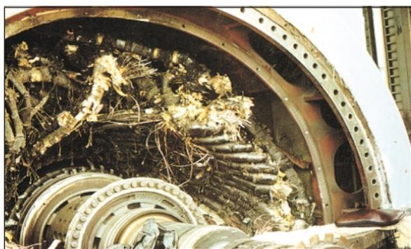
**Figure 15.** Catastrophic retaining ring failure
