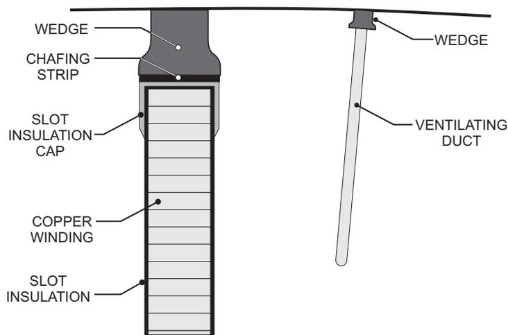
**Figure 5.** Indirect cooled coil slot
