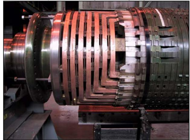
Fig. 1 Typical field endwinding
