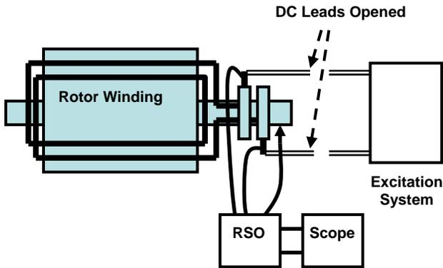
Fig. 9 Measuring setup for a "spinning RSO" test
