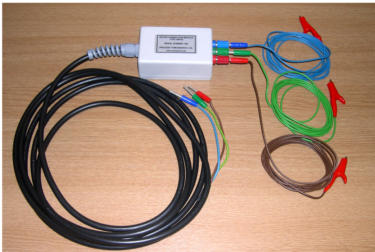
Figure 2.2 Rotor test leads and connection module
