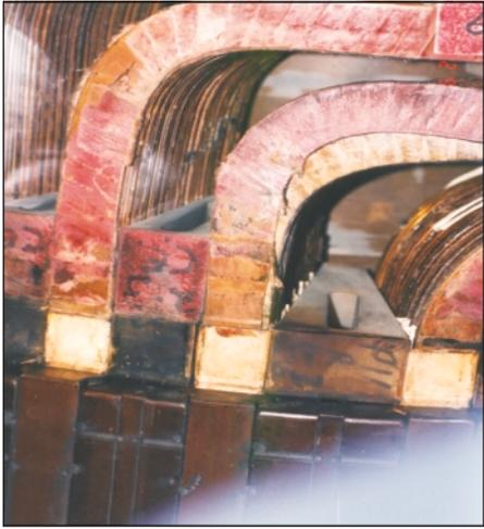
**Figure 13.** Moderate copper distortion
