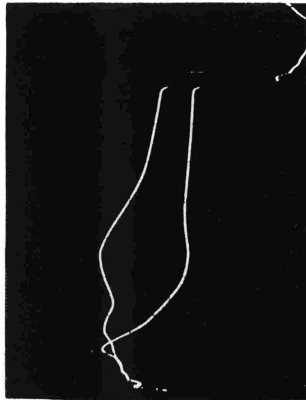
(a) Short circuit to rotor body at end of 5th slot coil (16 coils in winding).
