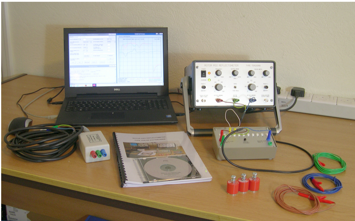
Figure 6.1(a) The TDR200 RSO Rotor Reflectometer measurement system in digital mode
