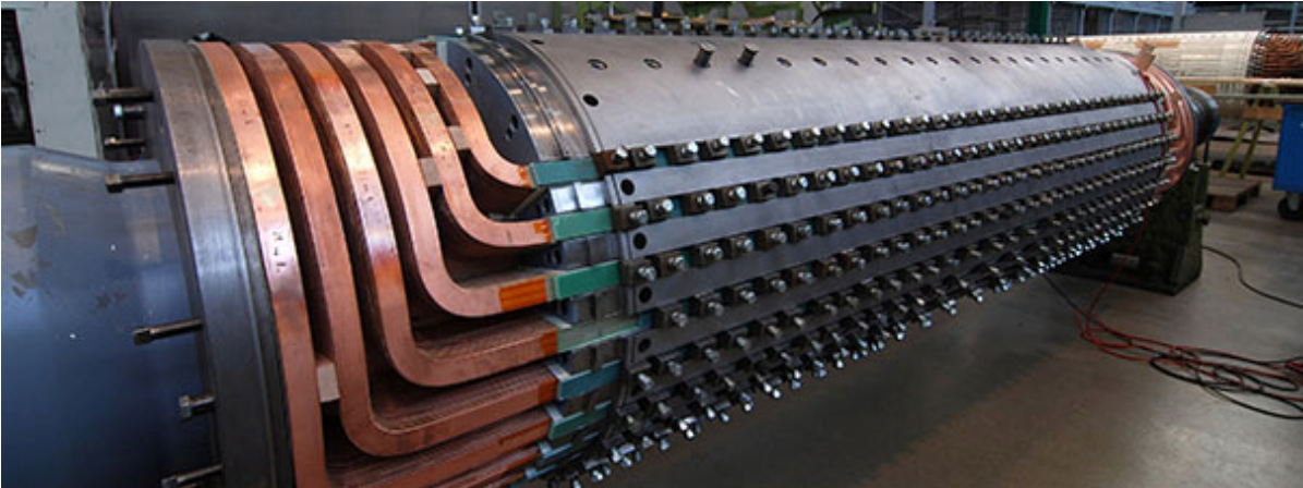
Figure 2.6 Cylindrical rotor winding with end (collector) rings removed
