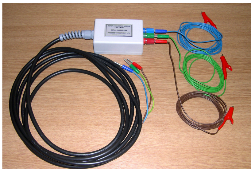
Figure 9.1 Rotor test leads and connection module
